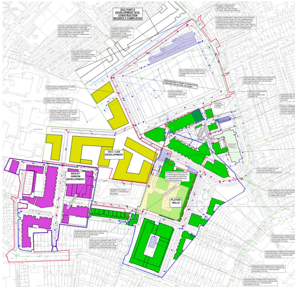
Figure 7.7 Proposed Combined Sites Drainage Strategy Plan (Extract from Engineering Drawing Set)
