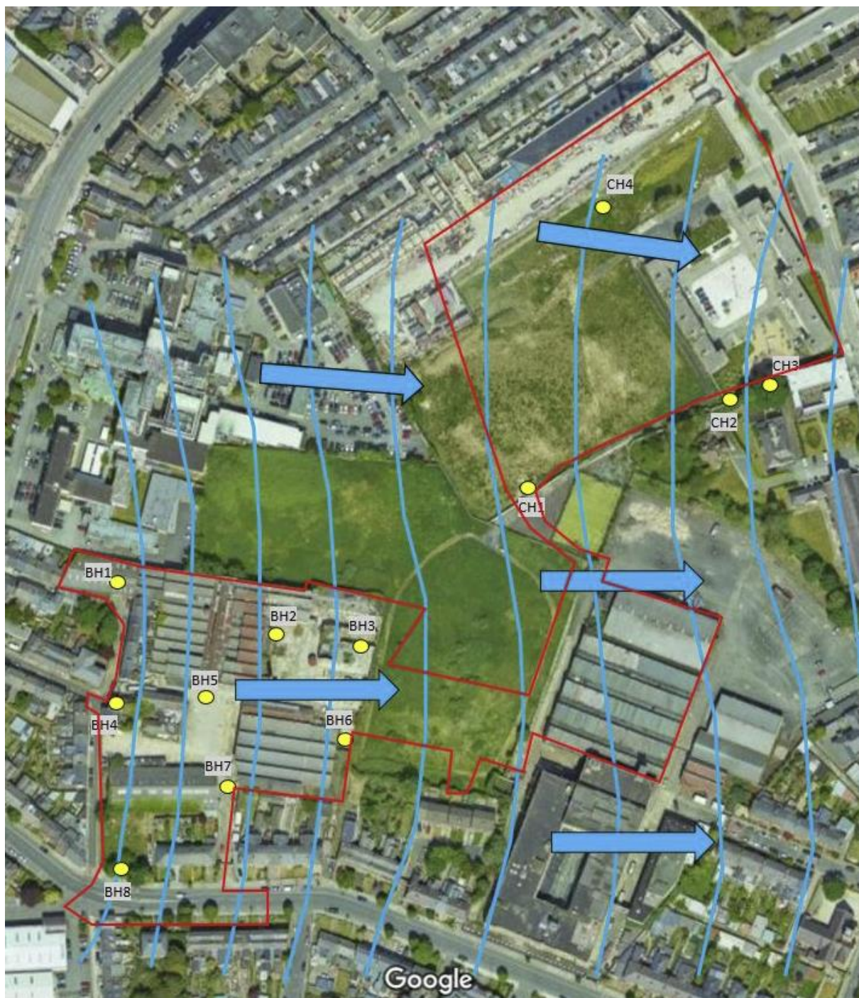
Figure 9.7 Groundwater Flow Direction
