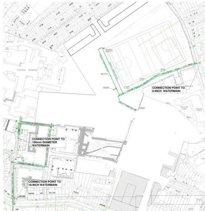
Figure 7.2 Proposed Potable Water Supply Connection Point (Extract from Engineering Drawing Set)
